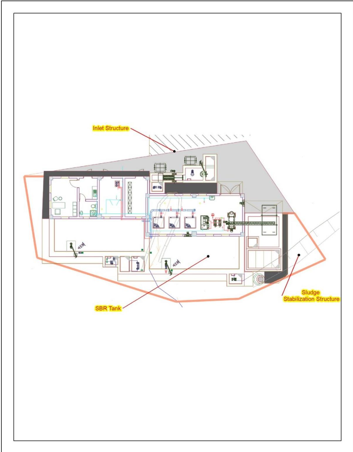
Figure III.3 Layout of Taskent WWT
