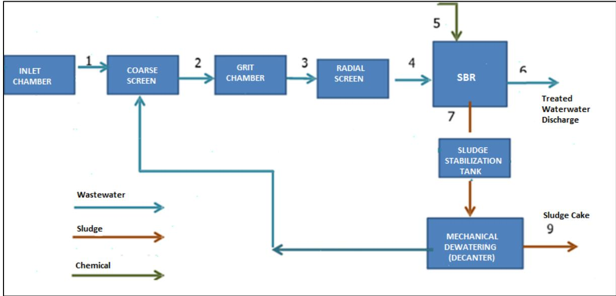
Figure III.1 Taskent WWTP Schematic Flow Chart
