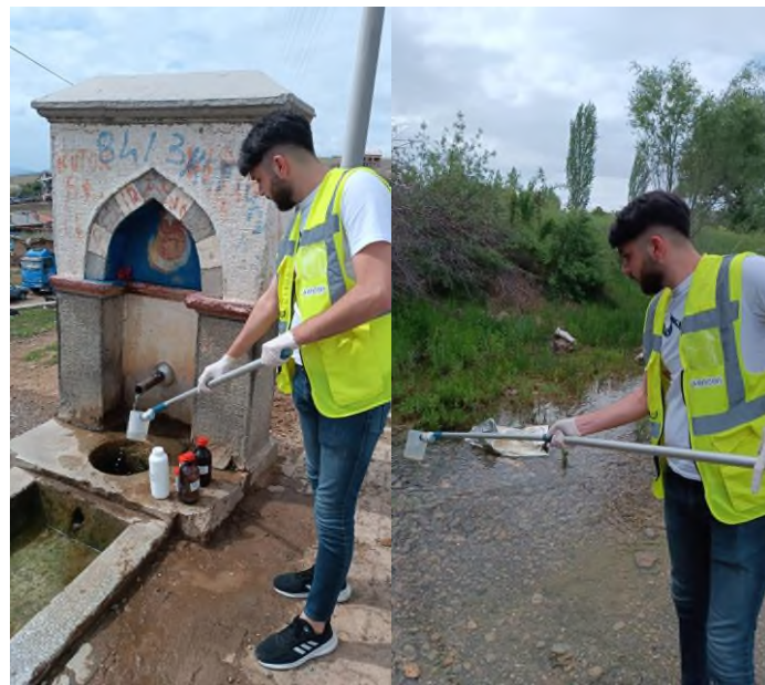
Figure 4-9 Groundwater and Surface Water Sampling
