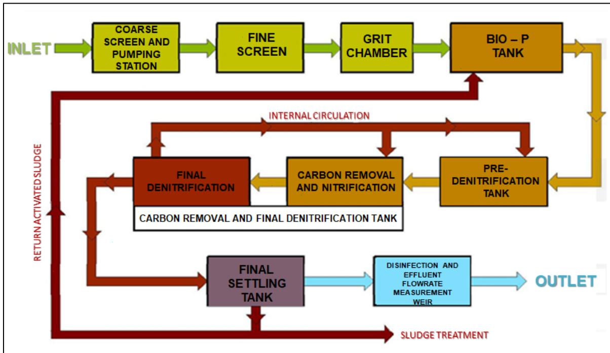
Figure III.1 Doganhisar WWTP Schematic Flow Chart
