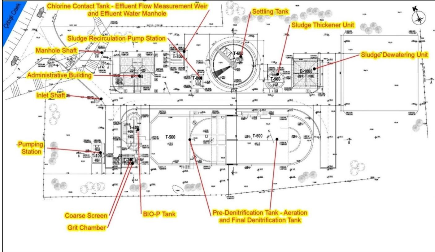
Figure III.3 Doganhisar WWTP Layout in 1:100 Scale
