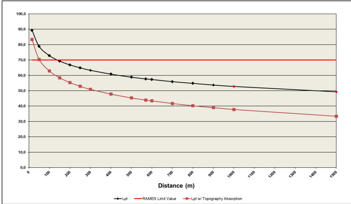
Figure V.3 Distribution of Noise Generated in the Project Area with respect to Distance
